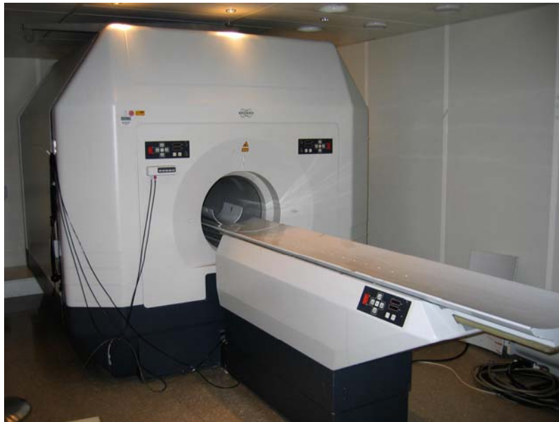
Figure 15. The 3 Tesla BRUKER Medspec 30/100 scanner at the Vienna MR centre of excellence was used for both anatomical and functional imaging in this study
